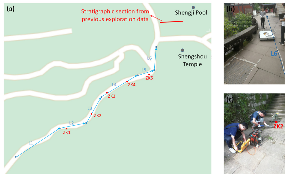
Figure 3. (a) GPR survey lines and borehole locations in the study area; (b) GPR L6 survey line data acquisition using a MALA 100 MHz antenna; (c) borehole televiewer image acquisition in borehole ZK2 using a JKX-4A borehole full-wall imaging system.
