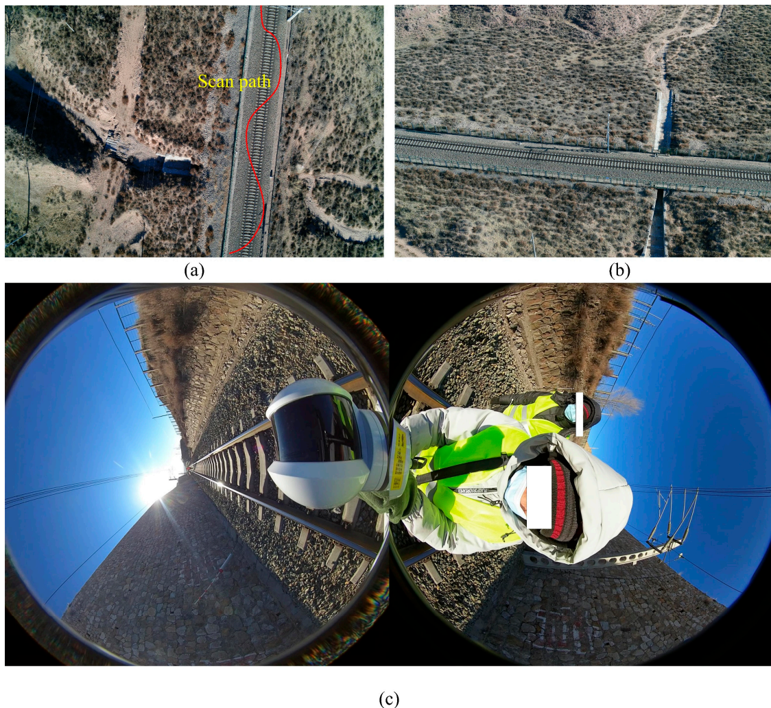
Figure 13. Data sources for Scene A: (a,b) railroad track; (c) scanning equipment.
