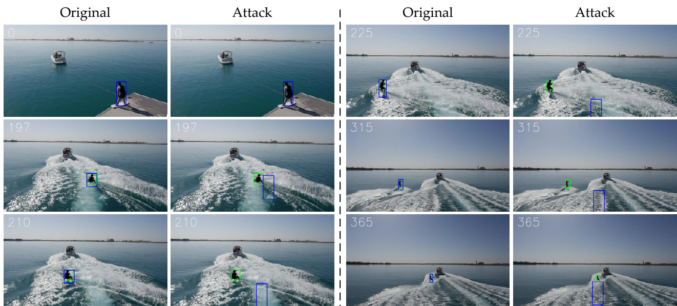
Figure 7. Visual comparison of the tracking results of the wakeboard video using SiamRPN++ (A) before and after being attacked by our proposed method. The green and blue boxes indicate the ground truth bounding box and the bounding box predicted by the tracker, respectively.
