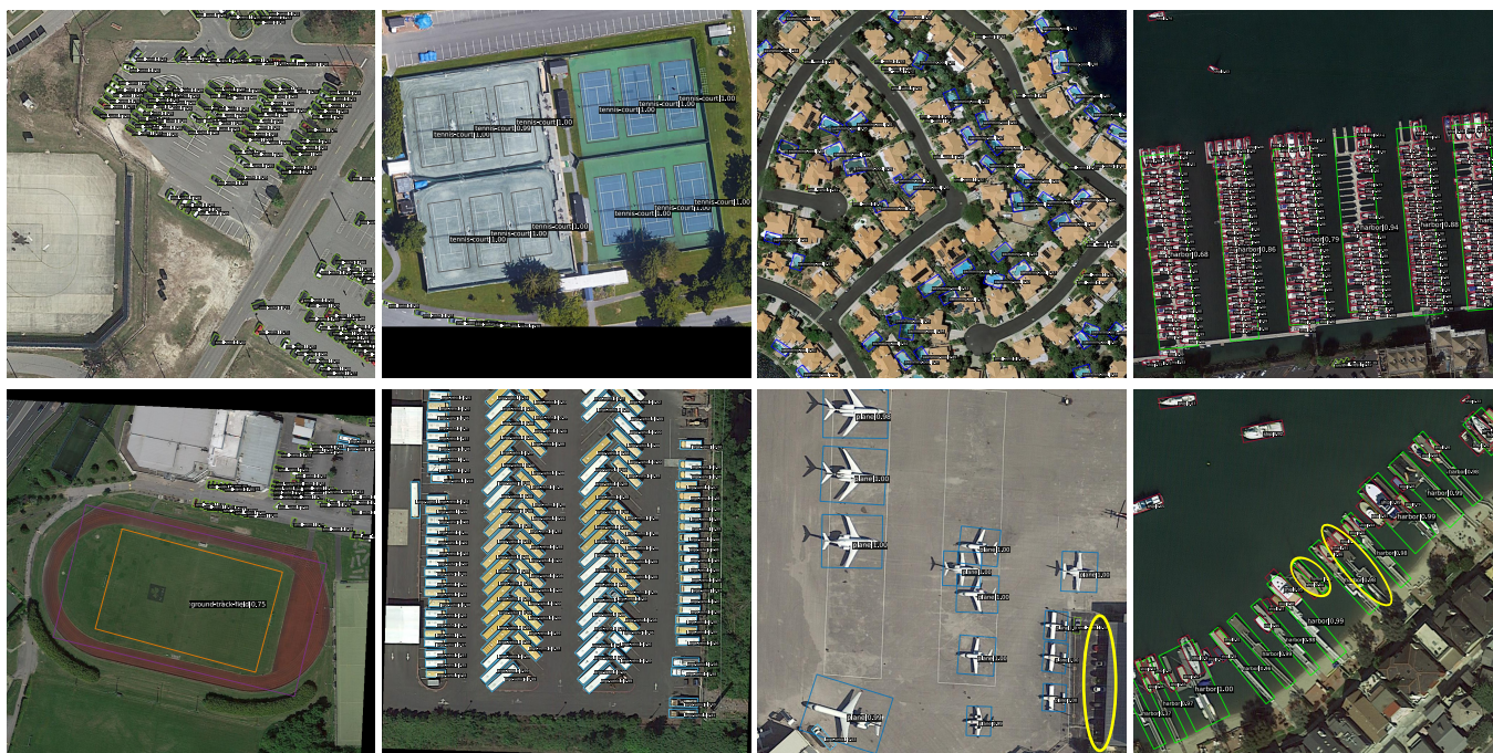
Figure 6. The visualization of the detection results on the DOTA dataset, the yellow ellipse means false detection or missed detection or inaccurate orientation prediction.
