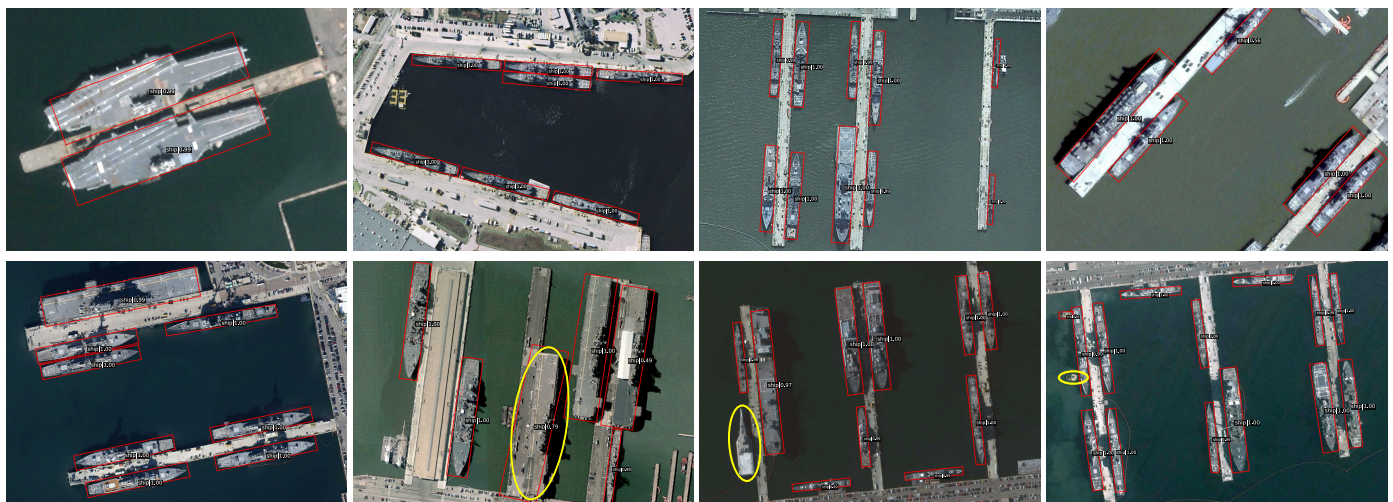
Figure 5. The visualization of the detection results on the HRSC2016 dataset, the yellow ellipse means false detection or missed detection or inaccurate orientation prediction.
