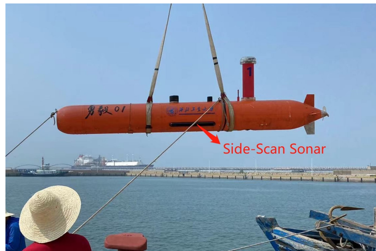
Figure 6. The AUV and the SSS utilized in the experiment.
