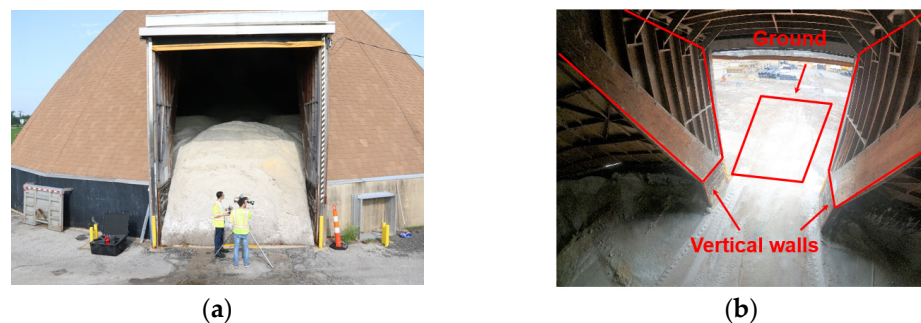
Figure 22. Demonstration of planar features near the entrance of a salt dome facility: (a) tripod-mounted SMART system stationed near the entrance and (b) wall/ground features.
