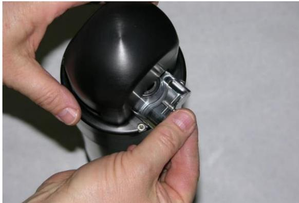
Fill chamber with (clean, particle-free) water, **optical quality filtered Milli-Q water (18.2°)** is ideal.
