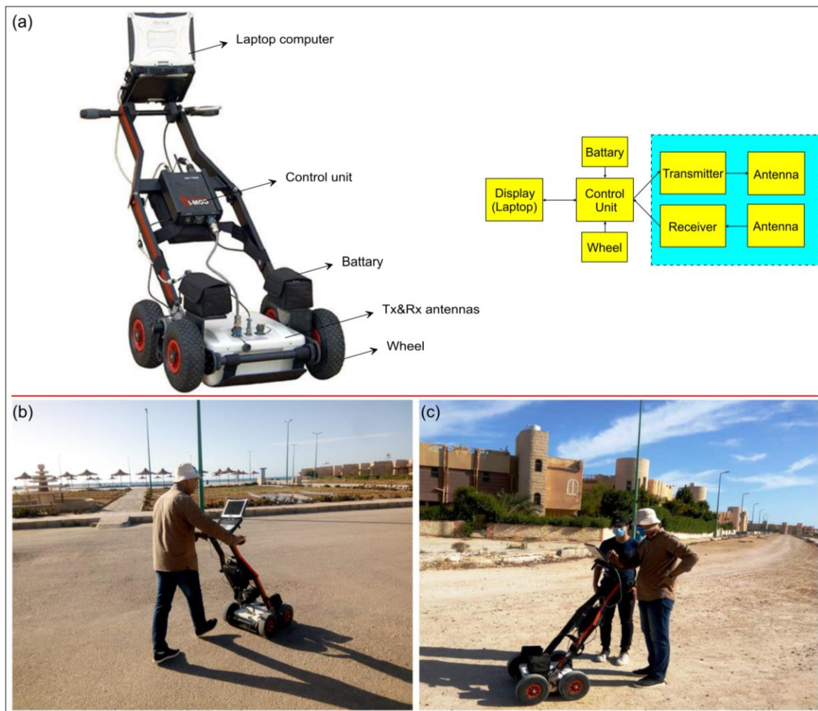
Figure 6. RIS Hi-MOD-IDS georadar system (a) and field photographs during the GPR data acquisition (b,c).
