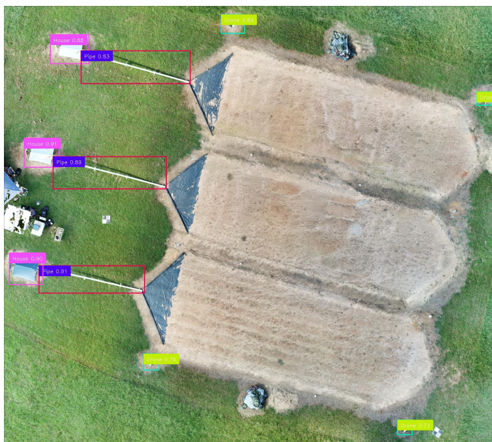
Figure 6. Reference objects detected from the ortho-photo. The object marked as the drone class are the black/white ground targets.
