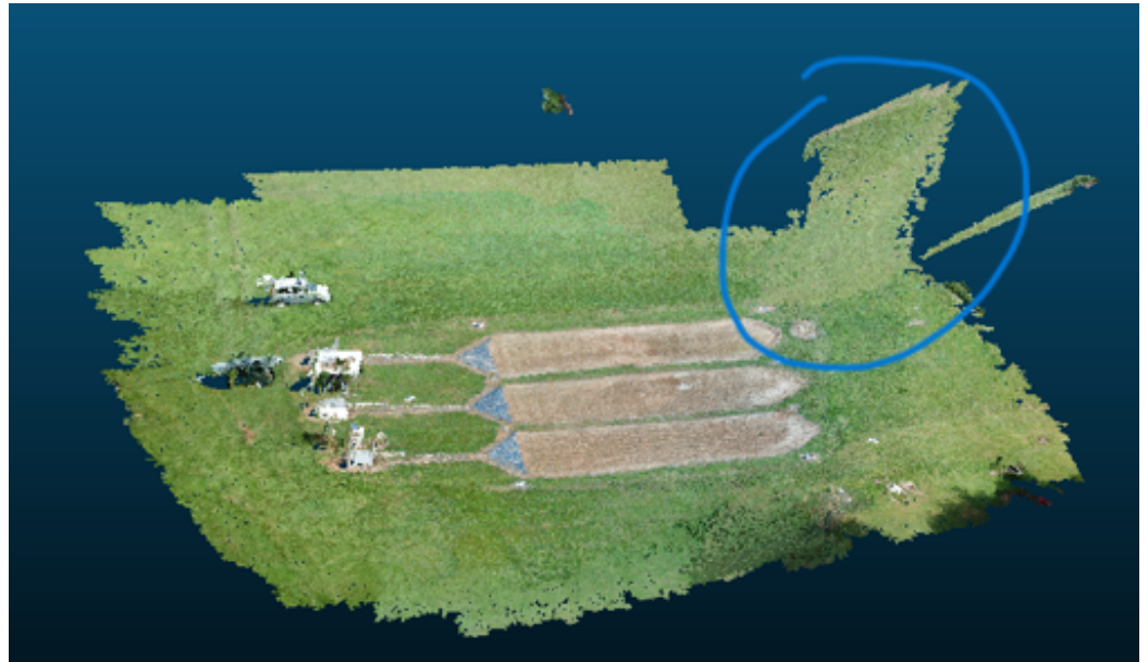
Figure 3. A point cloud of our test area generated by Pix4D with a dense noise set (the part circled in blue) because of bad photo quality.
