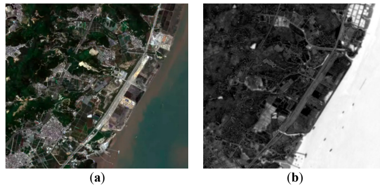
Figure 4. RGB image and MNDWI result. (a) RGB color composite image, and (b) MNDWI.
