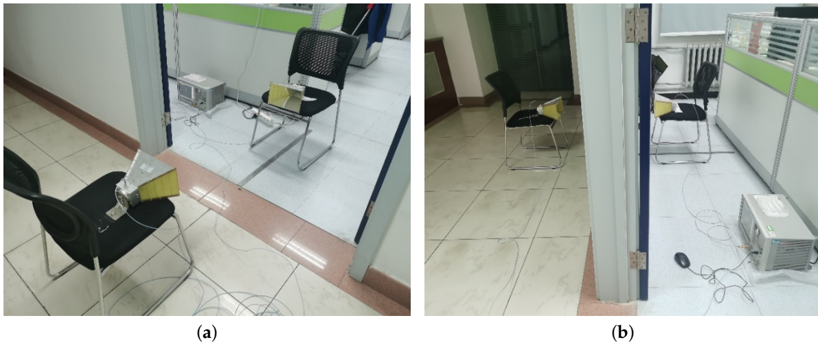
Figure 13. Penetration experiment scene: (a) The two antennas were placed opposite each other. (b) Two antennas penetrated the wall.
