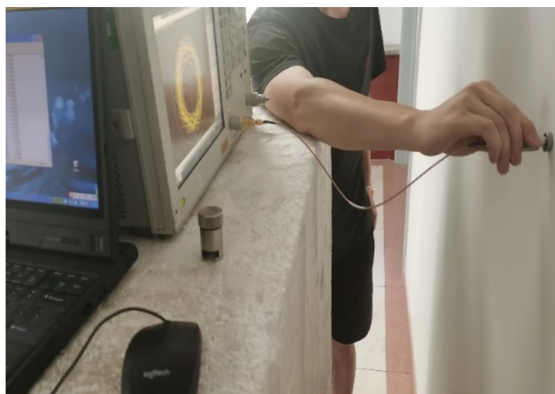
Figure 16. Experimental scene of dielectric probe detection.
