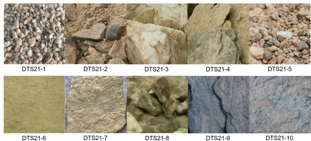
Figure 3. The 10 original-state rock samples used in this experiment.
