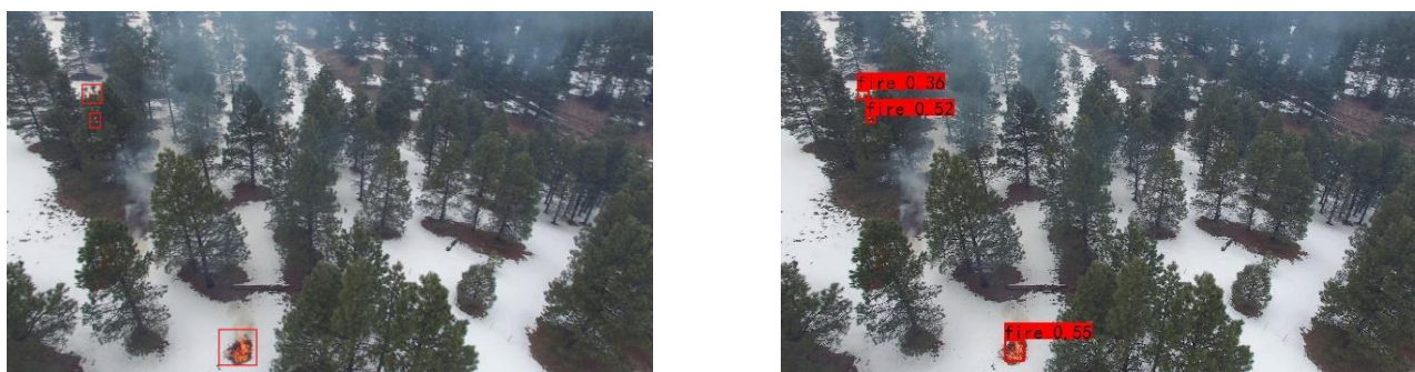
Figure 13. Detection results of FuF-Det on FLAME dataset (the left column is the original image with red boxes indicating the fire points, and the right column is the FuF-Det detection result).
