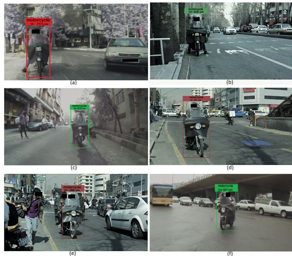
Figure 15. Motorcycle detection and range estimation results for the proposed MD-TinyYOLOv4 model which (a,d,e) are shown as a dangerous situation, and (b,c,f) are illustrated as a safe situation. Metric distances are also provided for each box.
