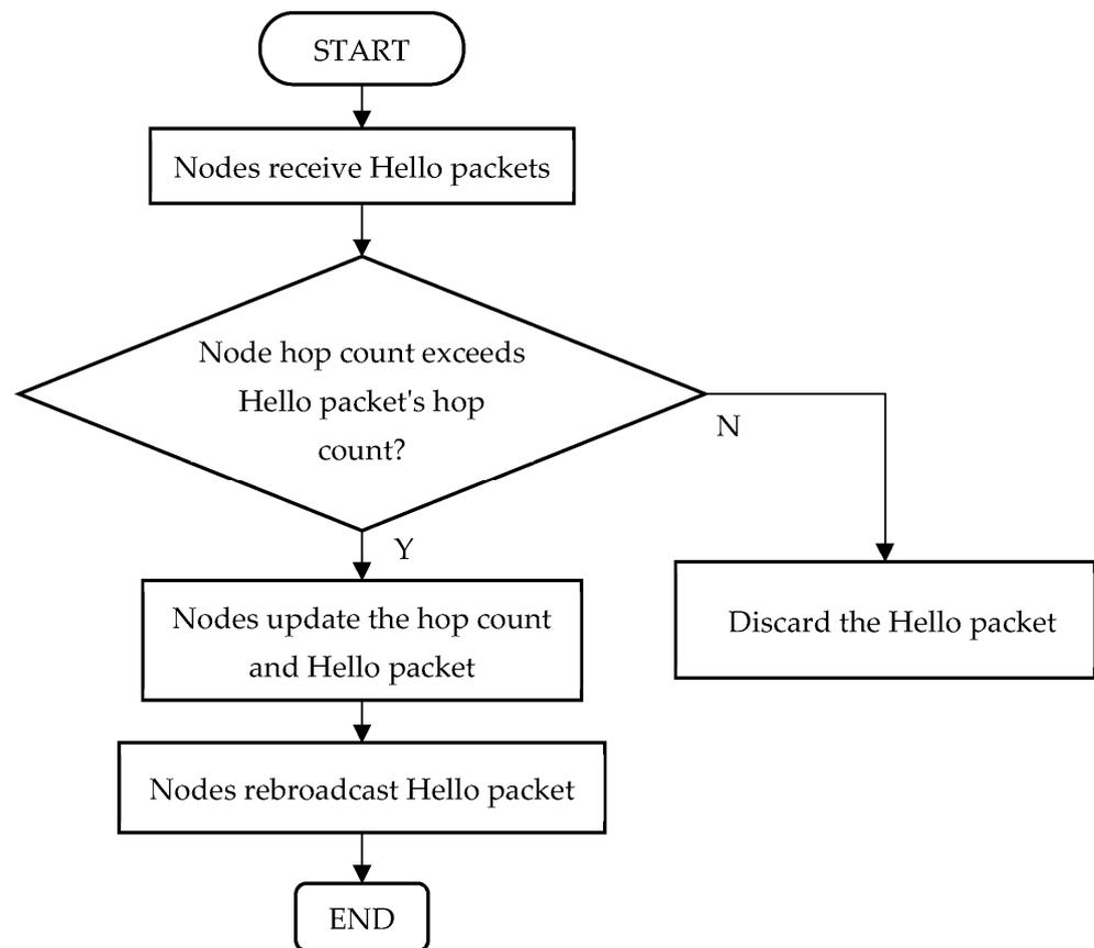
**Figure 2.** Flowchart for network initialization process.
