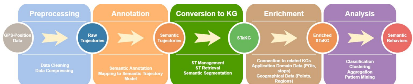
Figure 5. The STaKG pipeline (framework).
