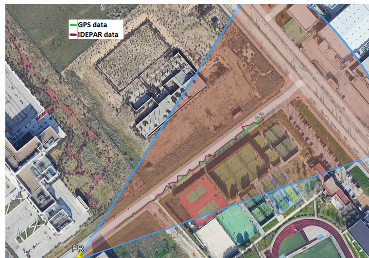
Figure 20. Estimated target trajectory with T_{int} = 500 ms versus GPS data in geographical coordinates.
