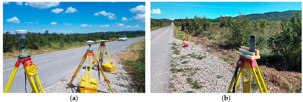
**Figure 4.** Test site in Črnotiče, Slovenia: (a) testing professional geodetic receivers in 2019; and (b) simultaneously testing smartphones and geodetic receivers in 2022.
