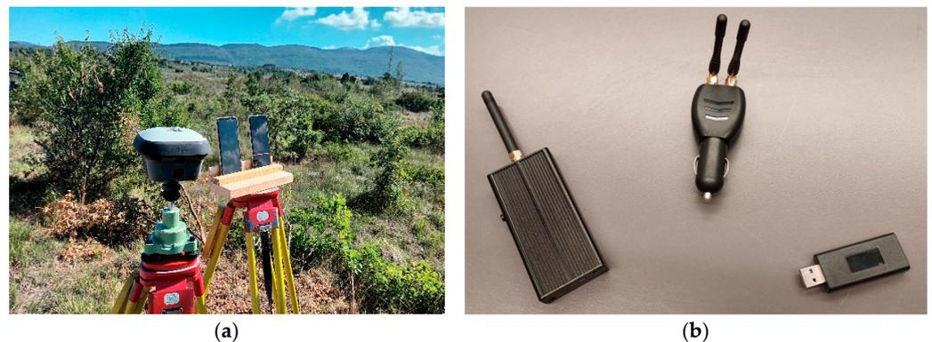
**Figure 1.** (a) Leica GS18 receiver and two smartphones setup; (b) jammers used in the experiment.
