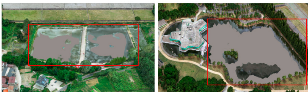
Figure 1. The effects of 3D reconstruction of water regions by UAV-based oblique photography technology, and the content in the red box corresponds to water regions in the real world.
