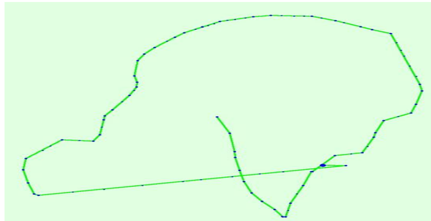
Figure 9. UAV flight route to gather oblique images. Lines represent the drone flight path; dots represent image capture positions on the flight path.
