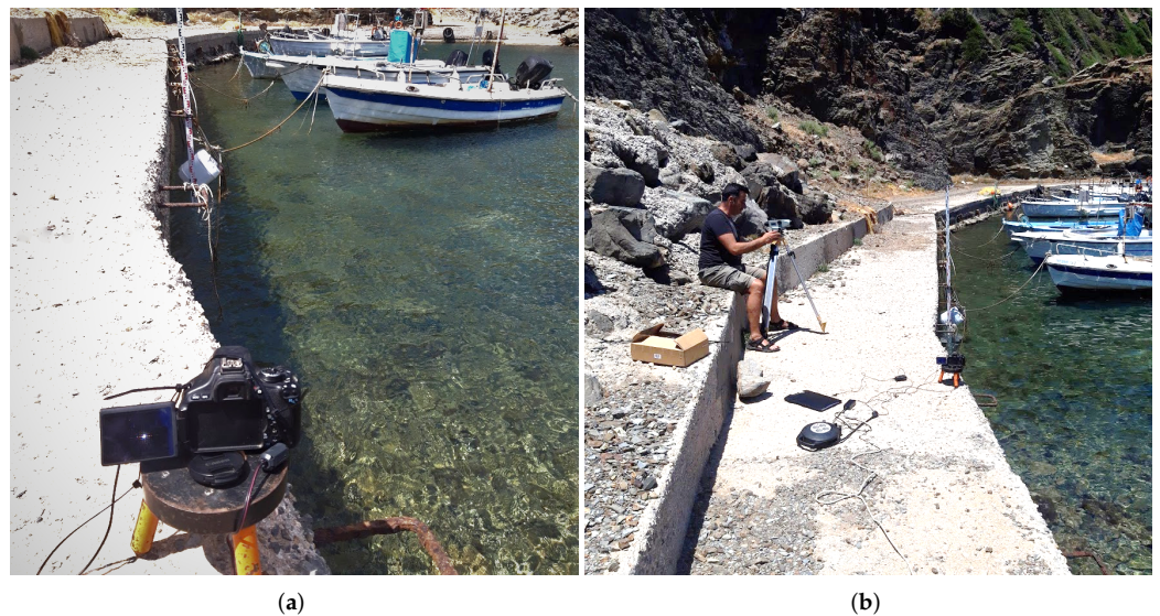
Figure 8. The setting for the execution of the video tide gauge experiment at RDK1 Cal/Val site (a) and the levelling survey carried out to tie tide pole measurements with water level measurements determined by tide gauges (b).
