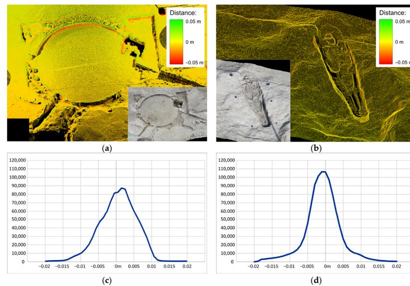
**Figure 6.** Comparison of TLS point clouds and 3D models obtained by photogrammetry: (a,b) distances from TLS points to 3D models; (c,d) frequency graphs of the cases (a,b).
