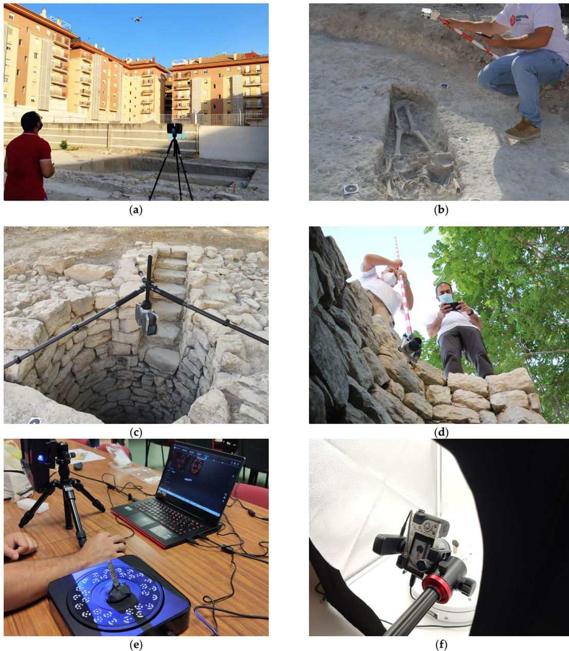
**Figure 4.** Examples of applications developed in this study: (a) RPAS and TLS acquisition (SL2–S4) of an excavation test; (b) CRP acquisition of a burial (SL3–S3); (c) TLS acquisition of a Roman well (SL3–S4); (d) CRP acquisition of a Visigoth burial (SL3–S4); (e) structured-light scanning of an artifact (SL4–S4); (f) V-CRP acquisition of an artifact (SL4–S4).
