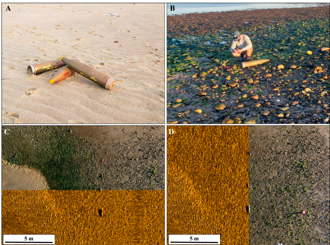
Figure 2. Intertidal survey areas. (A) Site 1, a sandy intertidal flat with a group of three 155 mm, wax-filled mortar shells. This group underwent no observable movement between one LT-HT-LT cycle based on RTK-GPS measurements. (B) Site 2, a mixed sand and gravel beach with many cobble-sized material. A single 155 mm, wax-filled mortar shell. (C) Site 2, horizontal sidescan data over the UAS imagery. Note the alignment of the second from the bottom target in both datasets. The bedforms in the lower left exhibit 12–15 cm spacing. (D) Site 2, vertical sidescan overlay over UAS imagery. Note the shadows in the lower two targets seen in the sidescan data.
