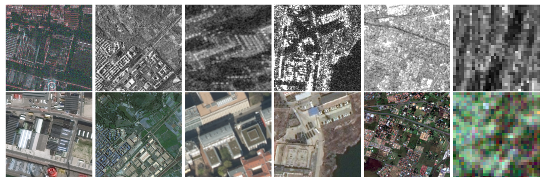
Figure 6. Sample patches of paired EO-SAR datasets. From (left) to (right): SN6-SAROPT, SAR2Opt, SARptical, QXS-SAROPT, SEN1-2/SEN1-2MS, So2Sat-LCZ42. The (top) row depicts the SAR images and the (bottom) row depicts the corresponding EO images. The shown image patches are resized to the same scale for visualization purposes.
