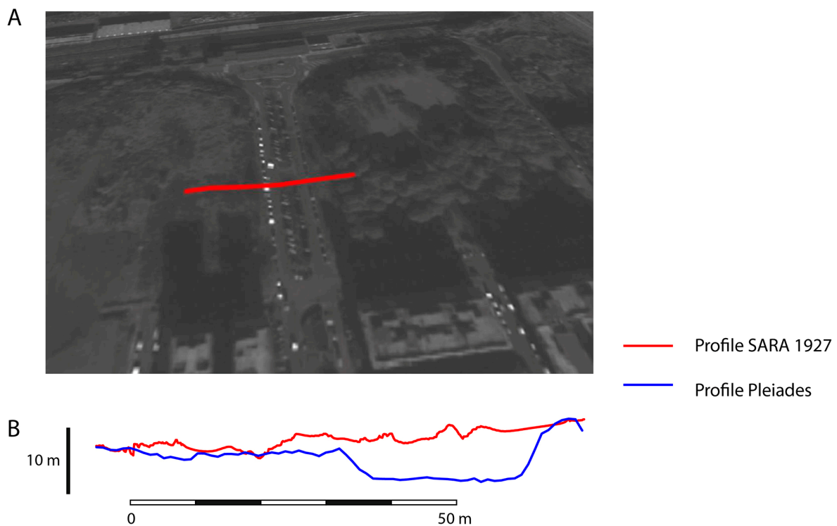
Figure 18. (A) 3D prospective view of the Pléiades-HR orthophoto on the DSM and of the profile (in red); (B) relative comparison of the profile shape extracted from the DSM SARA_1927 with the profile shape from DSM Pléiades—HR (stereopairs of January 2017).
