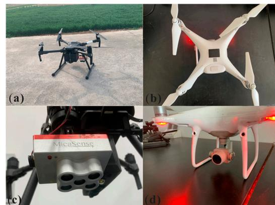
**Figure 3.** Drones for collecting data. (a) DJI M210, (b) DJI Phantom 4 Pro, (c) Red-Edge MX multispectral sensor, (d) RGB sensor.
