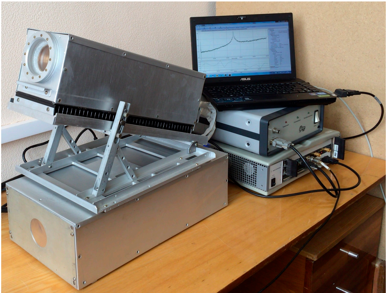
Figure 1. Spectroradiometer of the Institute of Applied Physics. The laptop display demonstrates the measured spectrum of downwelling atmospheric radiation at around \sim 110.836 GHz.
