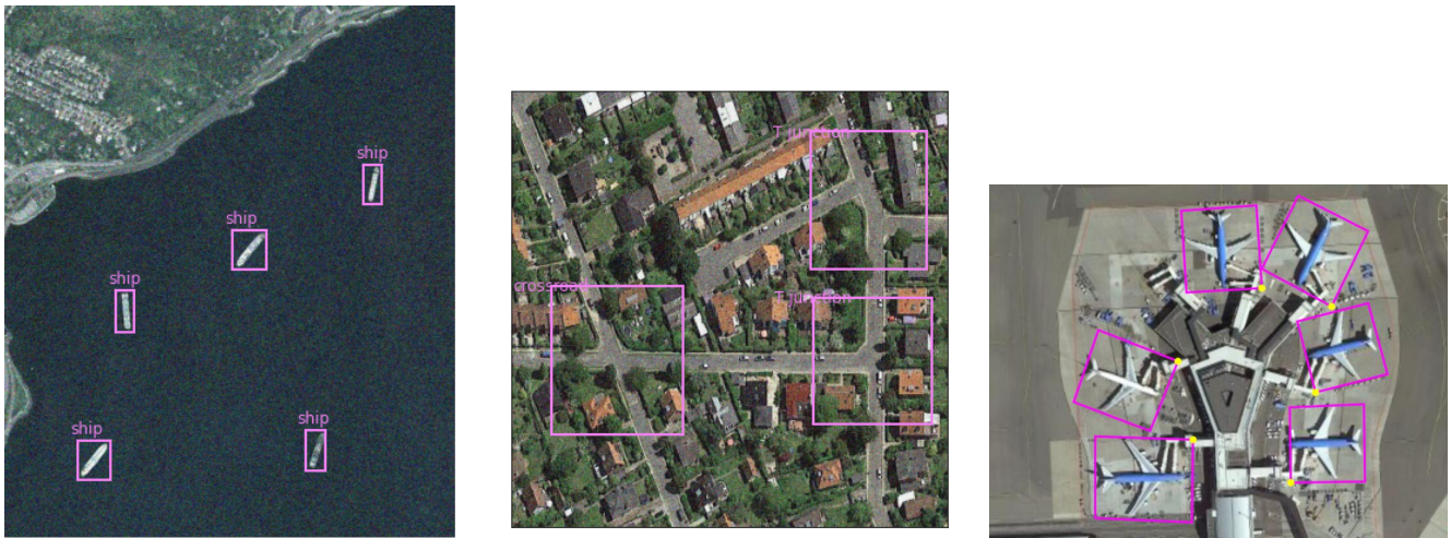
Figure 11. Example images with the predicted bounding boxes and object labels ('ship', 'T junction' and 'airplane', respectively) using a Faster R-CNN model.
