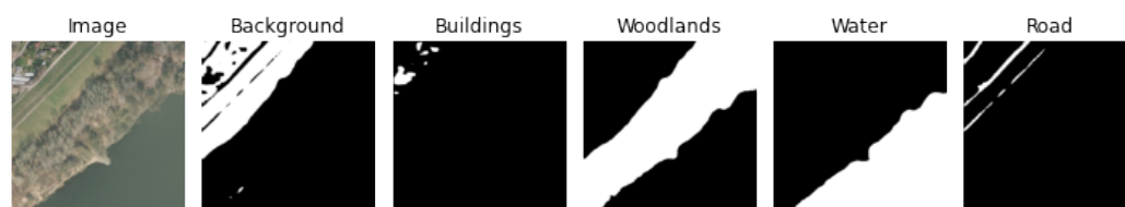
Figure A4. Example image with the predicted masks for each semantic label using the DeepLabv3 model.
