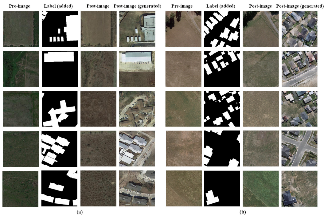
Figure 8. The generated building change detection sample pairs. (a) The generated sample pairs in LEVIR-CD. (b) The generated sample pairs in WHU-CD.
