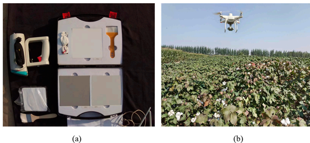
Figure 3. Remote sensing data collection. (a) An empirical line method was employed for each band (blue, green, red, red edge, and NIR), utilizing three reference reflectance panels (25%, 50%, and 75%). (b) Multispectral data were collected using a DJI P4M.
