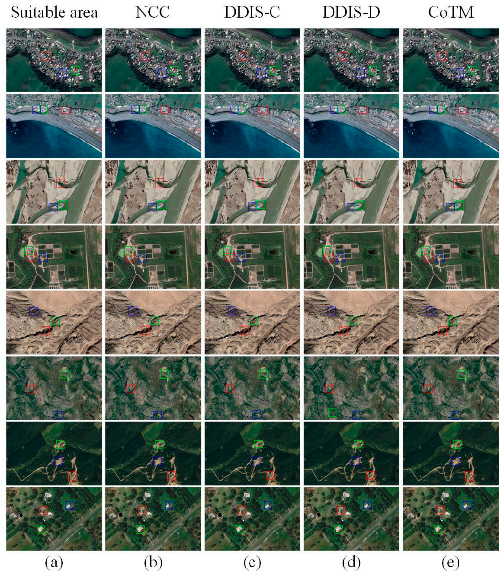
Figure 10. Matching results of different matching algorithms: (a) suitable area; (b) NCC; (c) DDIS-C; (d) DDIS-D; (e) CoTM. The green box is the No.1 suitable-matching area, the red box is the No.2 suitable-matching area, and the blue box is the No.3 suitable-matching area.
