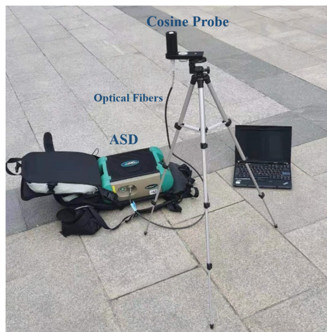
Figure 2. The outdoor variant illumination measuring device (IMD).
