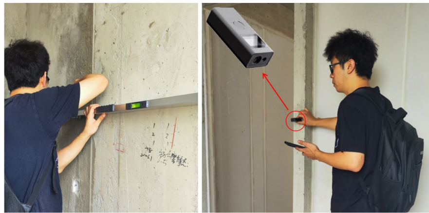
Figure 22. Manual measurements on the construction site.
