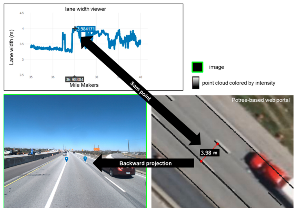
Figure 27. Illustration of a selected point in lane width plot (crosshair cursor) and the corresponding point pair in a LiDAR point cloud (connected by two red dots with a white-on-black label for the lane width), as well as the backward projected points (blue placemark), on an image.
