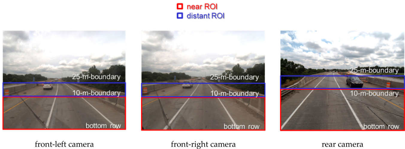
Figure 11. Near and distant ROIs for sample images captured by front and rear cameras onboard the PWMMS-HA.
