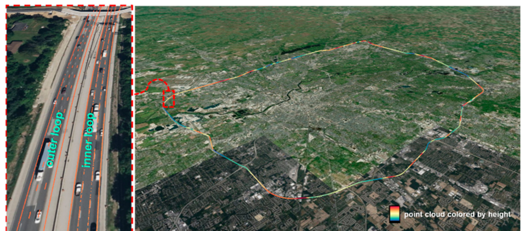
Figure 29. Illustration of the base map overlaid with lane marking point clouds and a zoom-in window (red dotted polygon) in the Potree-based web portal.
