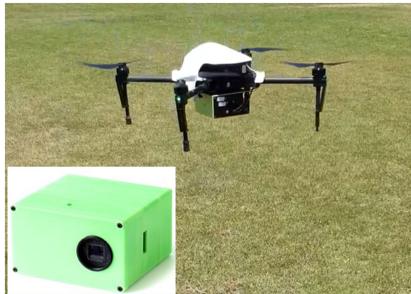
Figure 2. CoSpectroCam installed on Matrice 100 UAV.
