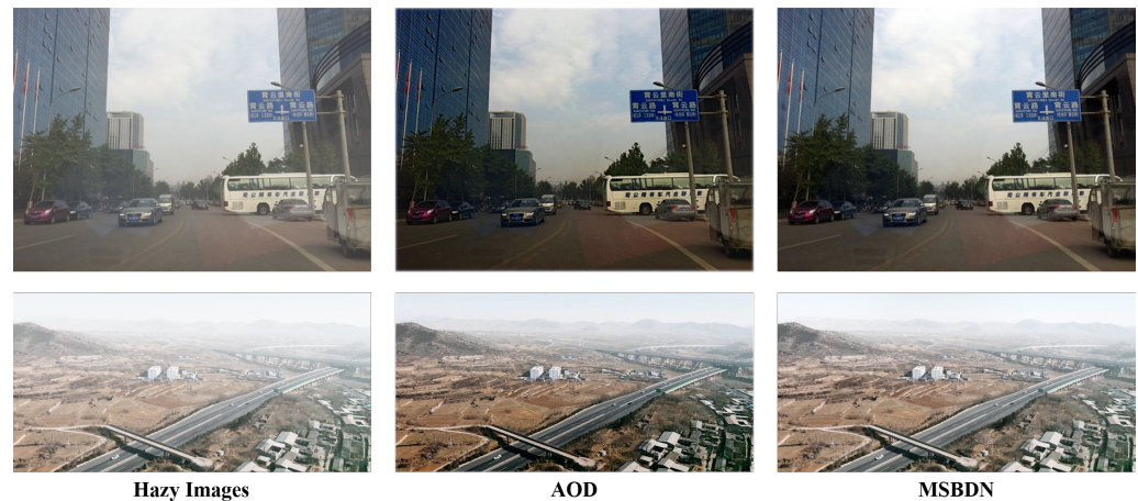
Figure 2. The dehazing effect on different scenes. The upper row is the normal perspective image from RESIDE, and the low image is the long-range perspective image from UAV-HAZE proposed by us. It can be seen that the previous dehazing methods work well on normal perspective but cannot restore the distant areas in long-range perspective images.
