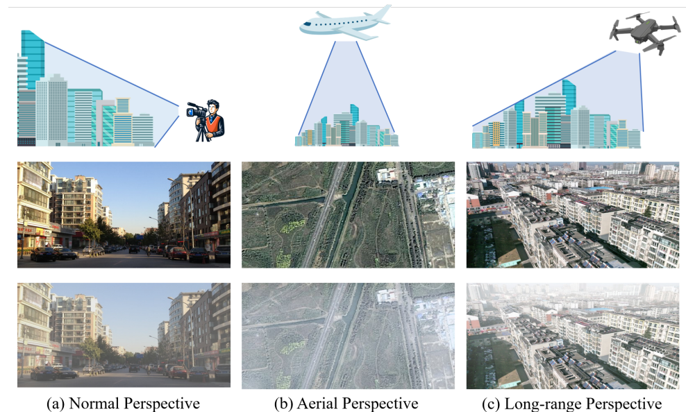
Figure 3. Different perspectives and captured clear and hazy images (from top to bottom: diagram, clear image, hazy image): (a) Normal perspective, captured from ground level, with a limited scene span leads to a relatively average haze density; images sourced from RESIDE [38]. (b) Aerial perspective, captured from high altitude, where depth variations can be ignored, resulting in haze density being less influenced by depth; images sourced from Sate1K [39]. (c) Long-range perspective, captured from low altitude with an inclined overhead view, providing a larger span compared to (a) and more details on surface objects compared to (b); the haze density varies significantly with depth changes; images sourced from UAV-HAZE. The drawn materials in the image are sourced from Vecteezy ( https://www.vecteezy.com/ , accessed on 10 April 2024).
