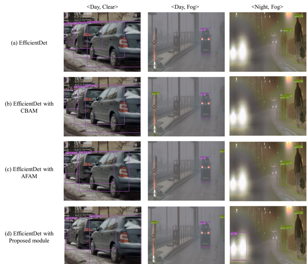
Figure 9. Object detection performance qualitative results. (a) Only camera feature-based object detection result; (b–d) camera–LiDAR fusion-based result; (b) with CBAM module; (c) with AFAM module; (d) proposed module using reinforcement learning and genetic algorithm.
