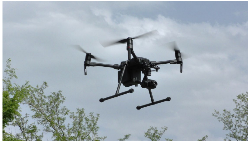
Figure 2. The UAS utilized in this work (Matrice 210 and Zenmuse-XT2).
