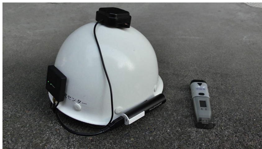
Figure 3. GNSS equipment (F9P) attached to a helmet (left) and a thermohygrometer (right).
