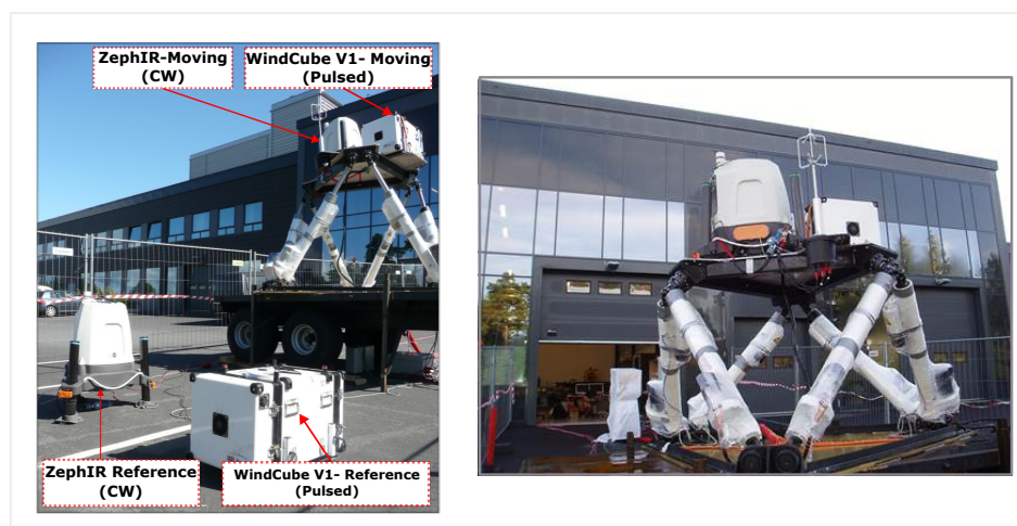
Figure 1. Lidars on the moving platform. A WindCube V1 and a ZephIR 300 were mounted on a moving Hexapod; reference lidars were placed 5 m west of the moving ones.
