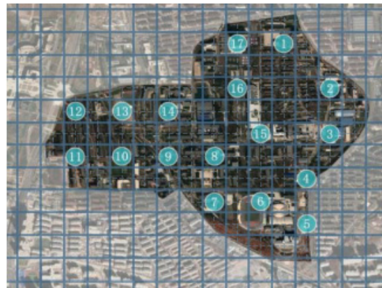
Figure 6. Layout of measurement units (The measurement points, that is, the numbers, are evenly distributed throughout the campus at a resolution of 130 m).
