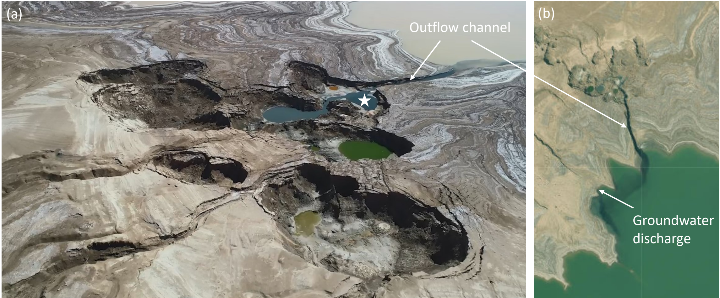
Fig. S6: Discharge sinkholes at the lower end of gully 10 and their outflow channel to the DS. For location, see Fig. 5. (a) Oblique drone photograph, February 7, 2019. White star marks the location of the first discharge sinkhole in 2015 (Figs. S4, S5). (b) 2023 aerial photo showing the outflow channel and groundwater discharge at the shoreline south of the channel.
