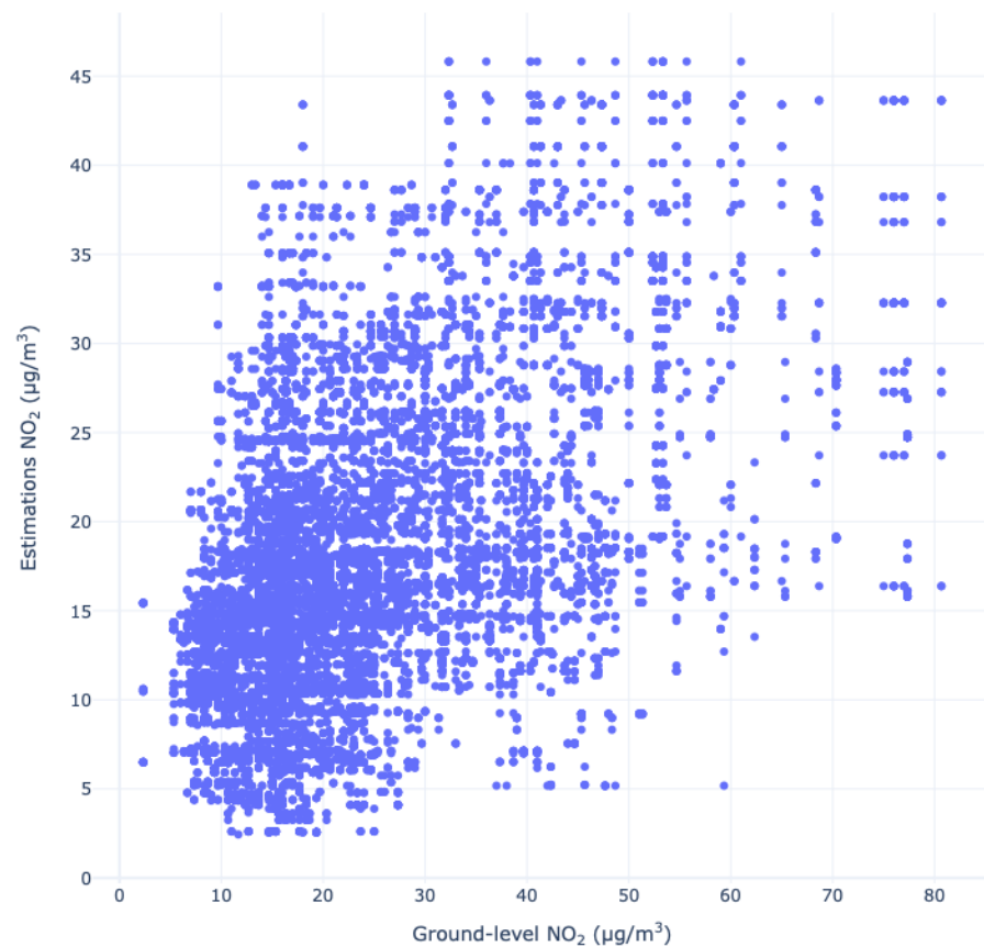
Figure 8. Scatter plot of NO 2 ground-level measurements from SIMAT and the model's estimations.
