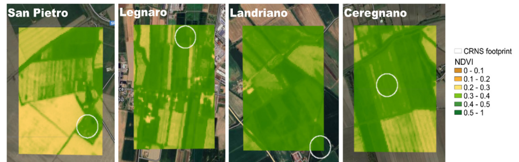
Figure 4. NDVI heterogeneity maps. Representation of the variations in vegetation vigor (median NDVI) within the areas covered by CRNS (white circles) and the SCATSAR-SWI footprint over the study period for four sites (maps were produced by https://earthengine.google.com , accessed on 15 January 2024).
