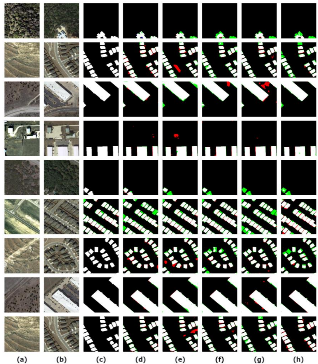
Figure 6. The building change visualization map: (a) T1 image. (b) T2 image. (c) Ground truth. (d) Our MDFA-Net. (e) BIT. (f) Change Former. (g) SNUNet. (h) USSFC-Net. Red indicates incorrectly identified pixels, while green indicates missed pixels.
