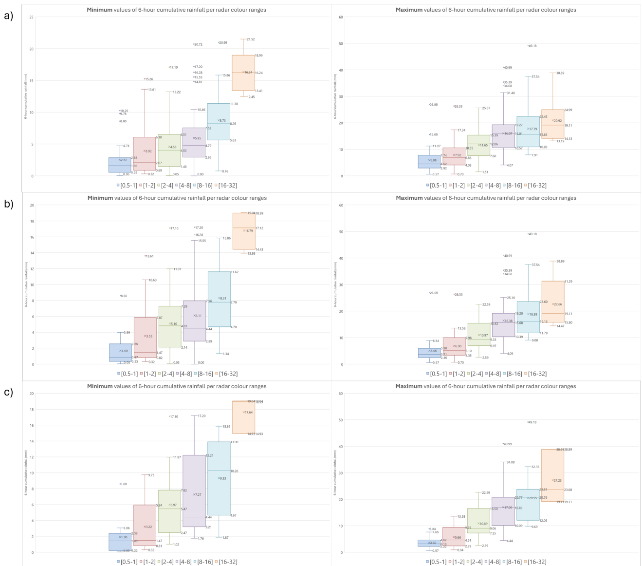
Figure 8. Minimum and maximum values of the 6 h observed rainfall for meteorological radar image colour ranges. Corresponding to (a) Satisfactory , (b) Good , and (c) Very good performance models.
