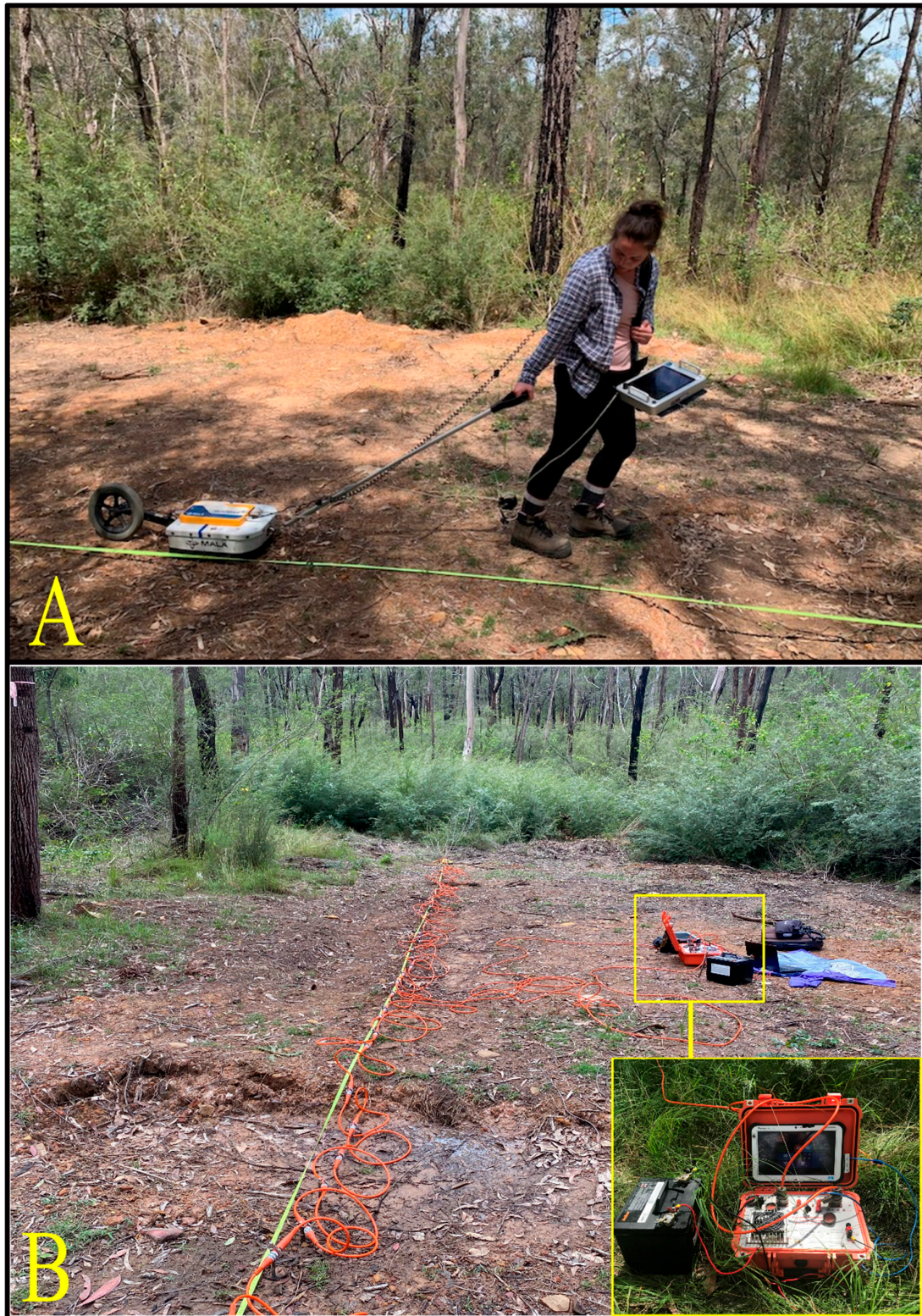
Figure 3. Geophysical techniques in use. (A) Mala X3M 500 MHz GPR system. This photo was previously published by Berezowski et al. [30] and is republished here with permission. (B) 64-electrode ZZ FlashRes 64 ERT system. This photo was partially published by Berezowski et al. [30] and is republished here with permission.
