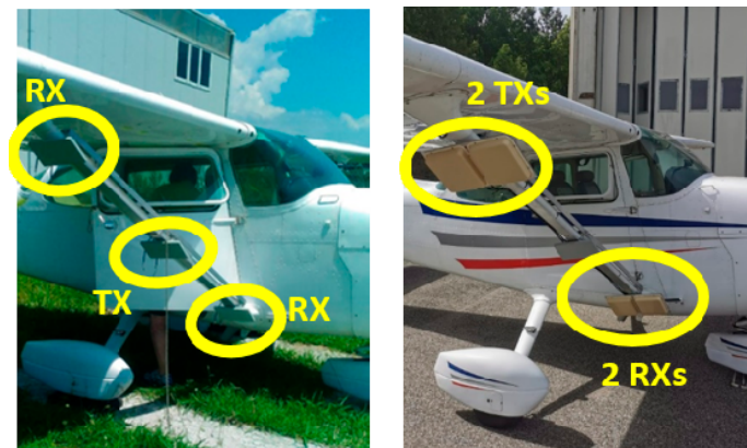
Figure 2. The X-band (left) and L-band (right) antenna layouts of the MIPS system mounted on Cessna 172 aircraft.
