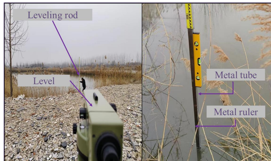
Figure 7. Measurement of the surface water level in underground coal-mining induced ground subsidence area using leveling surveying method (LSM).
