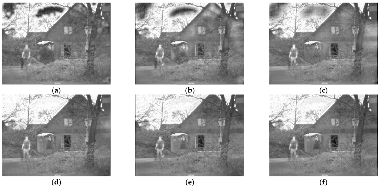
Figure 4. Fusion results of different decomposition levels in LP. (a) 1 level; (b) 2 level; (c) 3 level; (d) 4 level; (e) 5 level; (f) 6 level.
