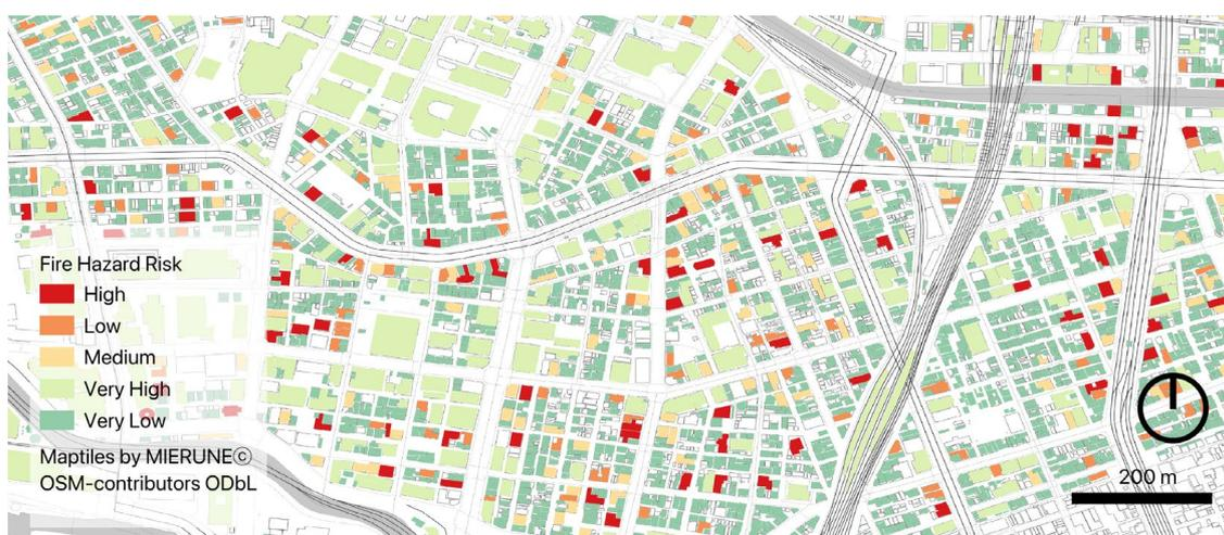
**Figure 14.** Prototype of the application in fire risk assessment (Tokyo, Japan).
